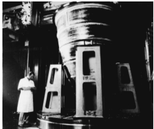
RA333 explosive forming die. Used in fabrication of the space shuttle engines.
