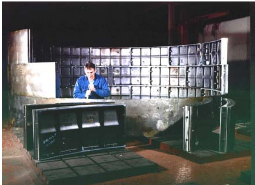
FIGURE 4 LUL tunnel linings fastened with Zeron 100 bolts.
