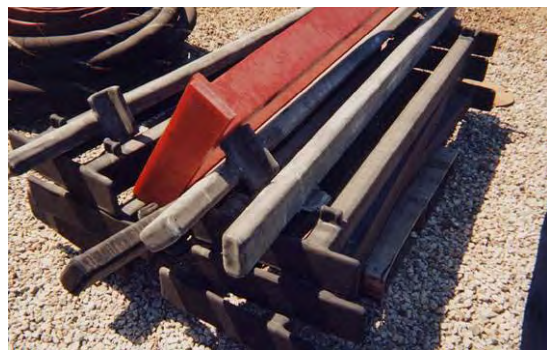
Figures 8 and 9: N08367 Alloy Box Beams replaced rubber coated steel beams (right).
