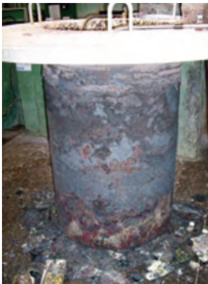
Fig. 7. Example of scaling happening on the outside of a salt pot after two weeks in service. The previous pot lasted over 15 years. The salt temperature was below 1300°F.
