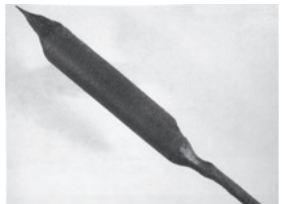
Fig. 2. 316L round-bar 3/4 inch in diameter exposed to 1800°F in air atmosphere. 316L is suggested to be used only to 1500°F due to scaling. In contrast, its melting point is 2540°F.
