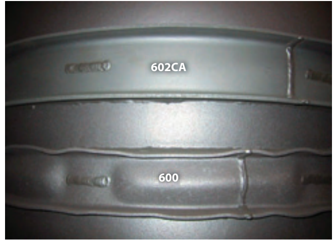
Figs. 5a. & 5b. Top of a coating retort made of 600 alloy with alternating reinforcement ribs of 600 and RA602 CA. The higher strength of RA 602 CA is evident in the close-up view. Retort wall temperatures are between 2000°-2100°F.
