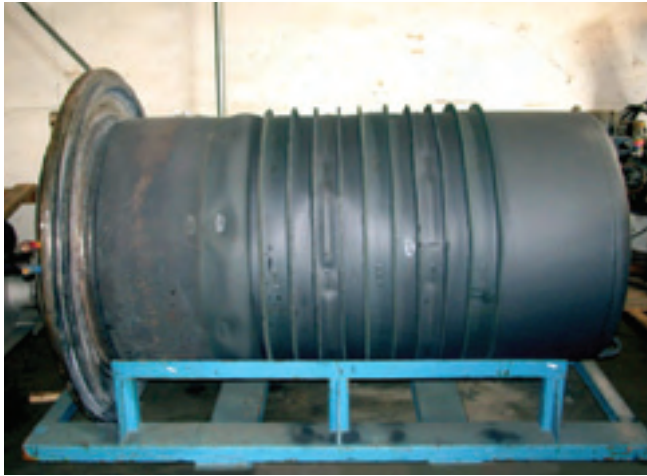
Figs. 5a. & 5b. Top of a coating retort made of 600 alloy with alternating reinforcement ribs of 600 and RA602 CA. The higher strength of RA 602 CA is evident in the close-up view. Retort wall temperatures are between 2000°-2100°F.
