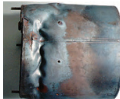
Fig. 8. This burner-can is a good example of what can happen when uneven heating occurs. In this case, flame impingement occurred during a low-fire condition.
