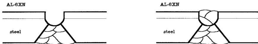
Weld the clad side with two or more layers of ERNiCrMo-3 weld wire or ENiCrMo-3 electrodes. Minimize dilution by using pulsed-arc GMAW (preferred), second choice FCAW or SMAW. A root pass with alloy C-22 wire or electrodes may be used, if desired, to counter-act dilution from the steel.
