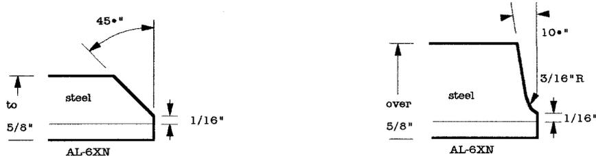
Tack the joint on the steel side using the same electrode as intended for the steel root bead. Finish welding the steel side.
