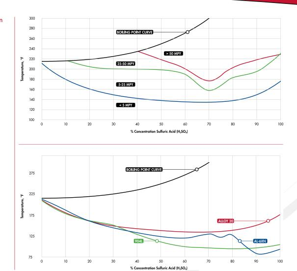
**Iso-Corrosion** Sulfuric Acid (< 5 MPY)
