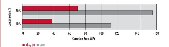
Alloy 20 Iso-Corrosion Sulfuric Acid
