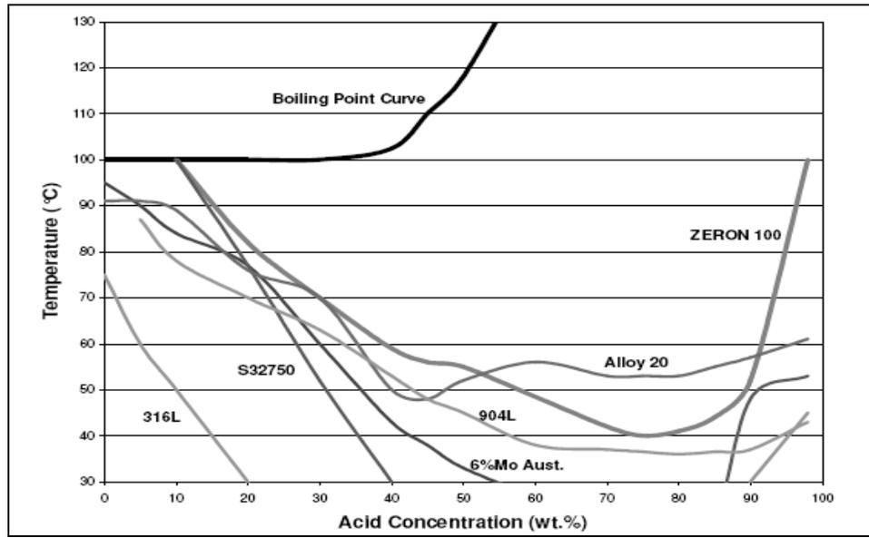
Figure 2 – Isocorrosion curve for various alloys in sulfuric acid. Corrosion curve represents a corrosion limit of 0.1 mm per year corrosion rate.
