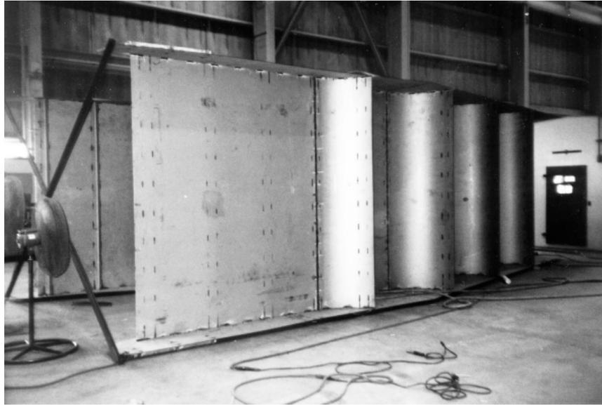
Figure 6 – AL-6XN was used for turning vanes installed in the flue stack at this Central Illinois Public Service Company Newton Power Station. This plant burns high sulfur coal hence condensation of a combination of acids and chlorides on the turning vane was a concern. AL-6XN was selected after testing.
