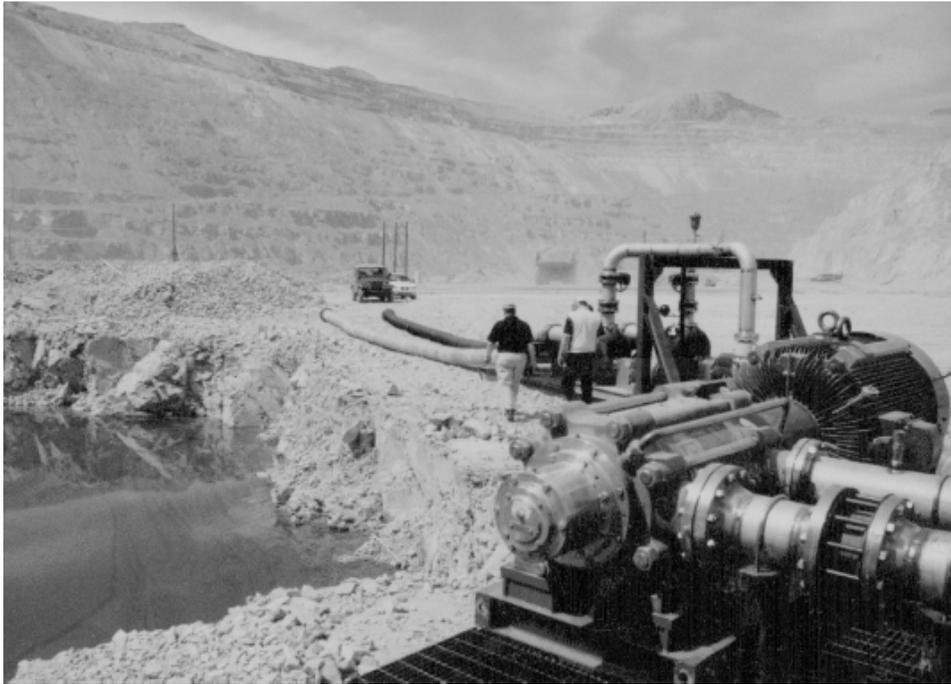
Figure 8 – ZERON 100 pump in a copper mine in the USA. ZERON 100 was used as it was subjected to sulfuric acid.
