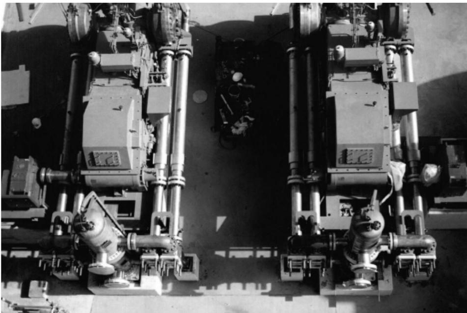
Figure 9 – ZERON 100 used for a nickel laterite-mining project in Australia. Pictured above are Geho positive displacement pumps made from ZERON 100.
