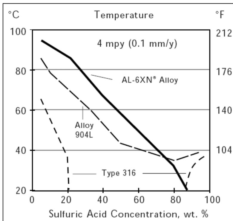
Figure 1 - Isocorrosion curve for various alloys in sulfuric acid. Corrosion curve represents a corrosion limit of 0.1 mm per year corrosion rate.
