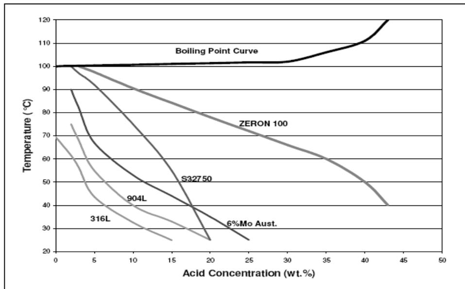
Figure 3 – Isocorrosion curve for various alloys in sulfuric acid plus 2,000 mg/l chlorides. Corrosion curve represents a corrosion limit of 0.1 mm per year corrosion rate.
