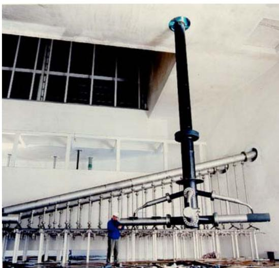
**Figure 2: N08367 Alloy Rotary Sparger**
