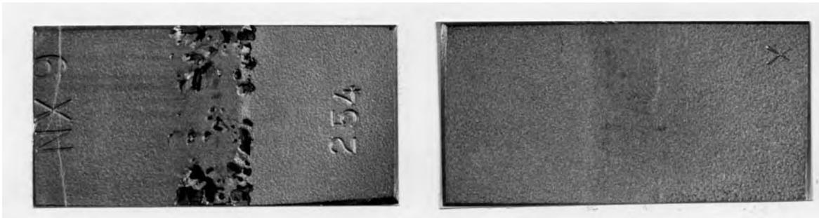
Figure 5 Sample condition after corrosion testing for 72 hours in 10%  $\text{FeCl}_3 \cdot 6\text{H}_2\text{O}$ , at 50°C (122°F). The autogenous weld is shown at left and the GTAW weld with 625 filler is at right.
