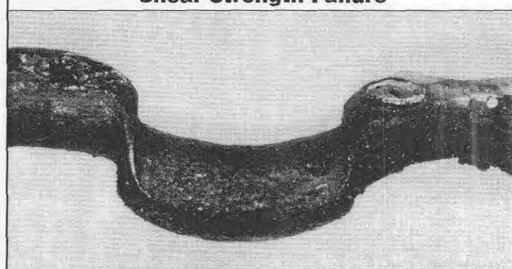
As a consequence of improper annealing, this belt pin lacks shear strength; its failure mode is called crank-shafting.
