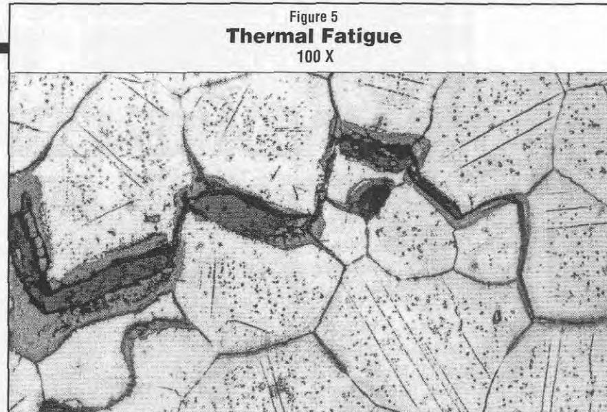
The direction of crack propagation in this 35Ni-19Cr alloy is from left to right.
