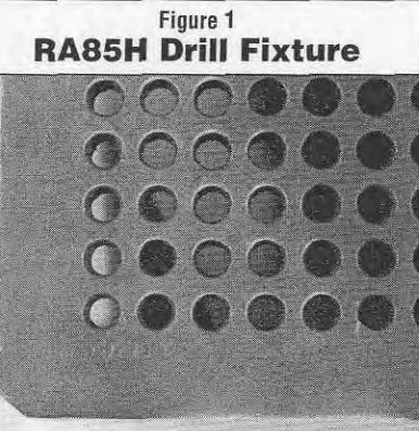
This RA85H drill fixture is used just above salt level in the fumes at a temperature of about 1500°F.
