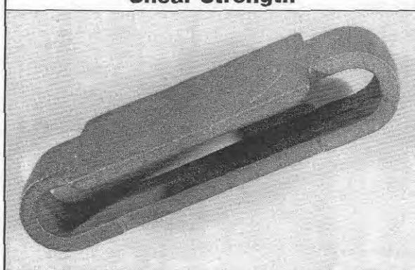
High temperature shear strength is important in this pin bearing link cast of 35 Ni 17Cr .4C alloy because as part of a cast-link furnace belt it must bear shearing loads.
