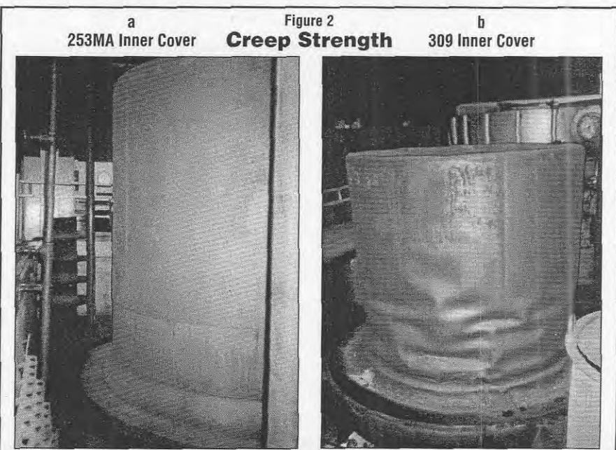
Operating at 1700°F, the nitrogen-cerium strengthened RA253MA in Figure 2a shows no deformation, but the 309 stainless inner cover shows marked creep buckling.
