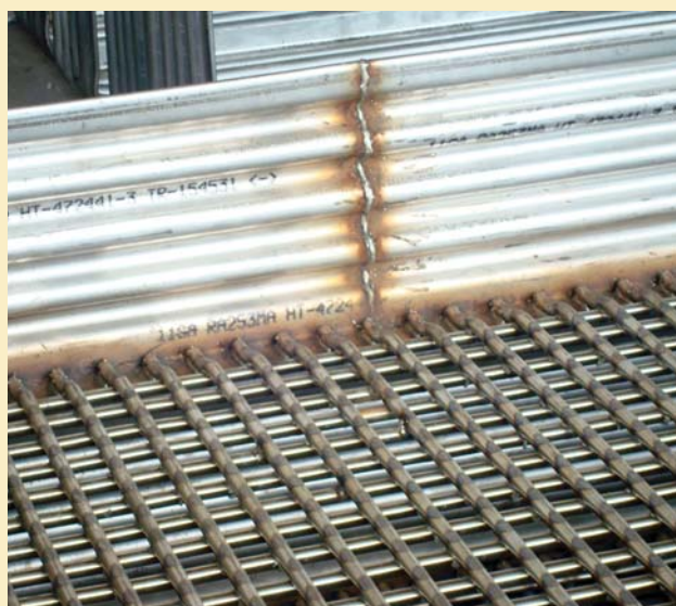
72" x 72" RA 253 MA corrugated boxes made of 11ga sheet with 5/8-inch diameter round-bar grids used for an isothermal heat treatment at 1600°F
