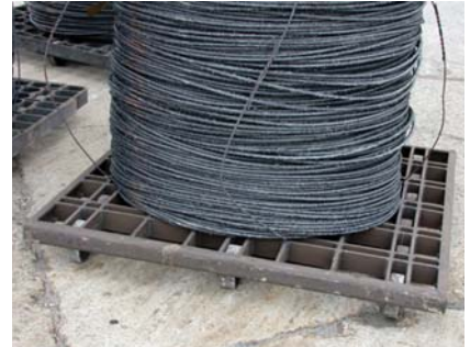
Fig. 2. Fabricated RA330 tray
