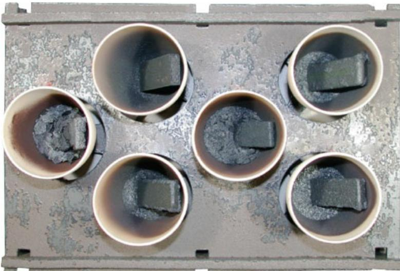
Fig. 2. Oxidation testing fixture, 2,880 hours at 2200°F.
