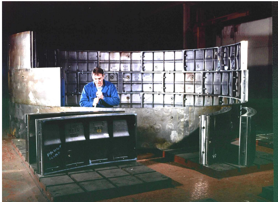
FIGURE 4 Cast Z100 rings being checked for dimensional compliance.
