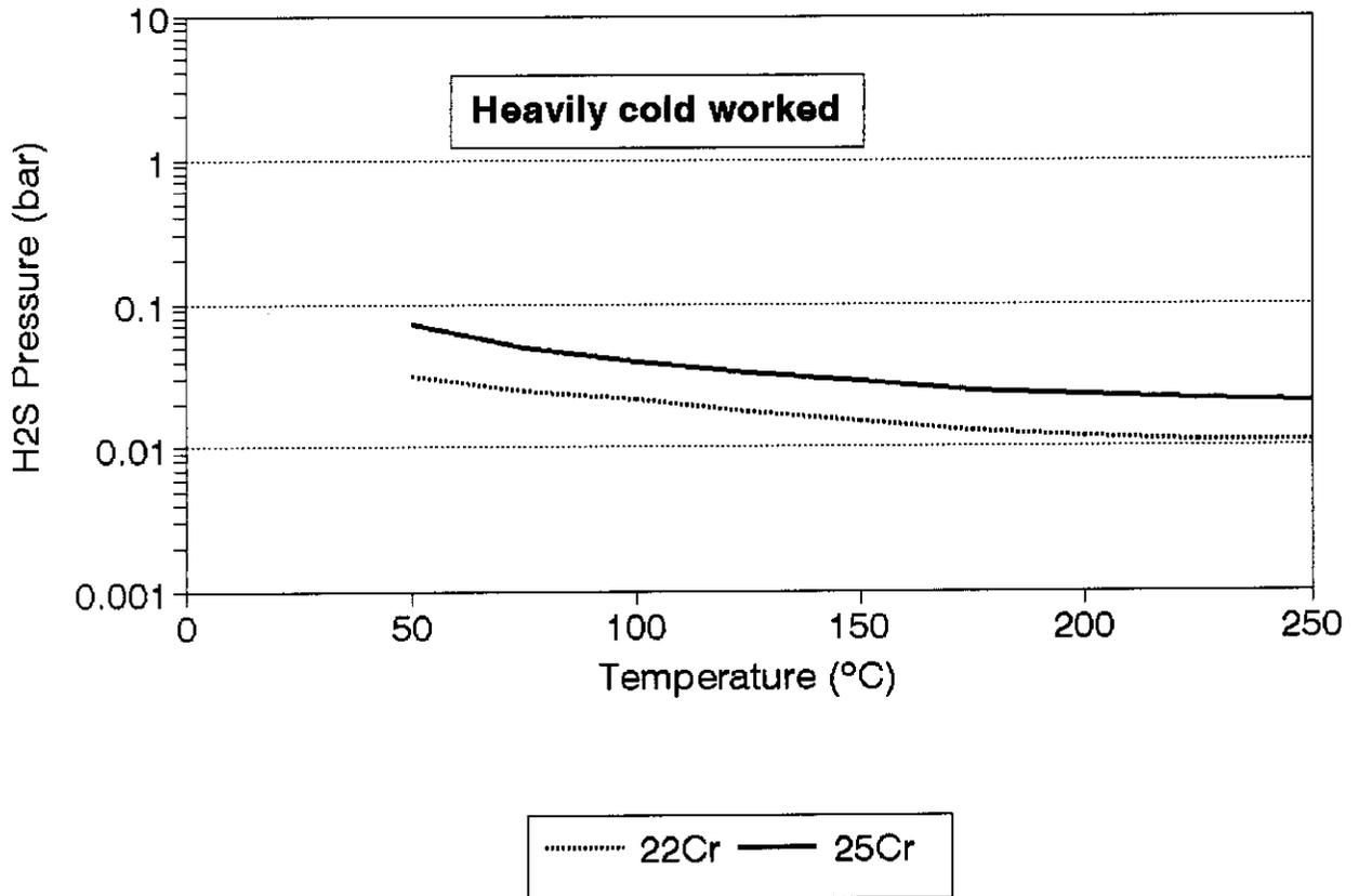
**FIGURE 3 SSCC tests on cold-worked proprietary super duplex at pH3 to 4**
