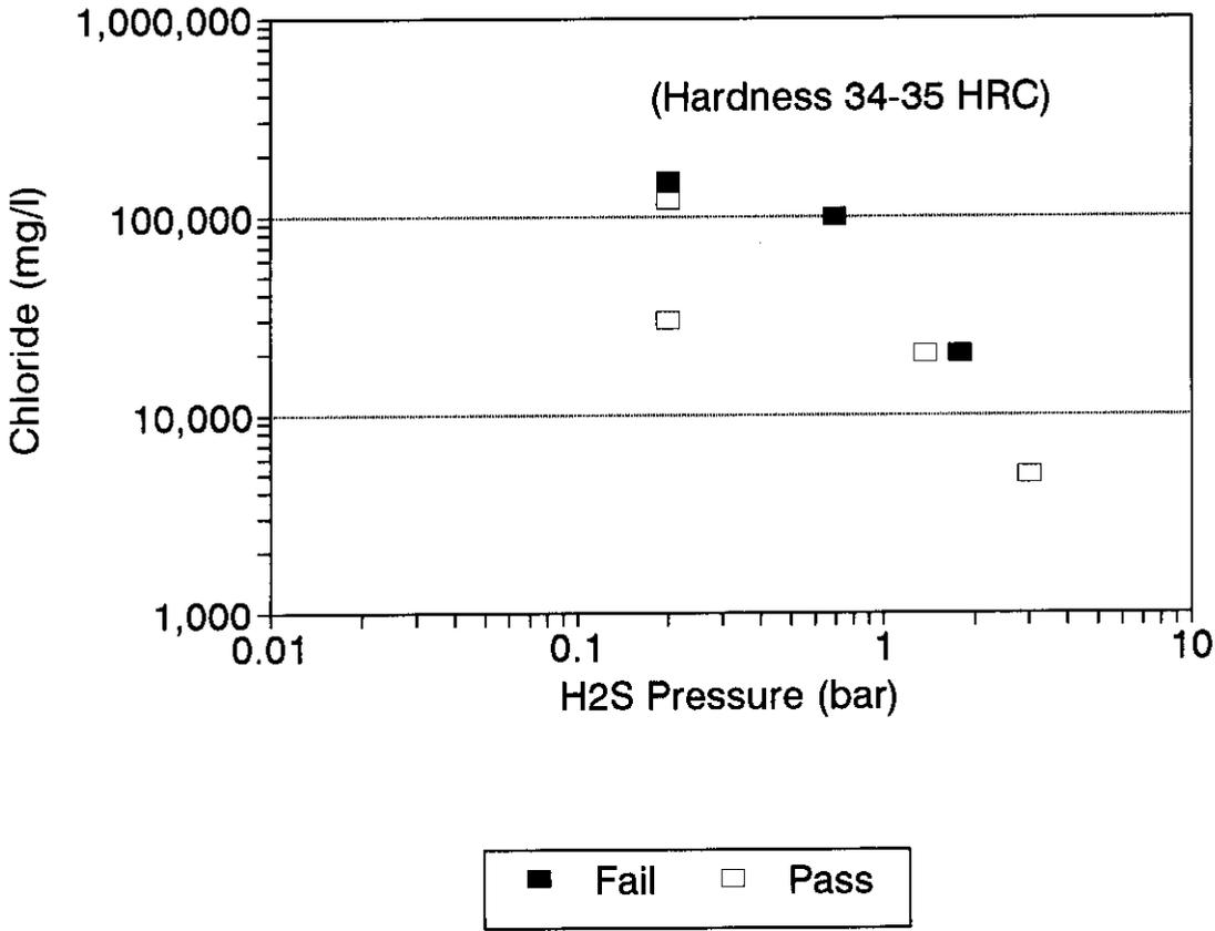
**FIGURE 4 Comparison of proprietary SSCC data with NACE MR0175 for UNS S32760**
