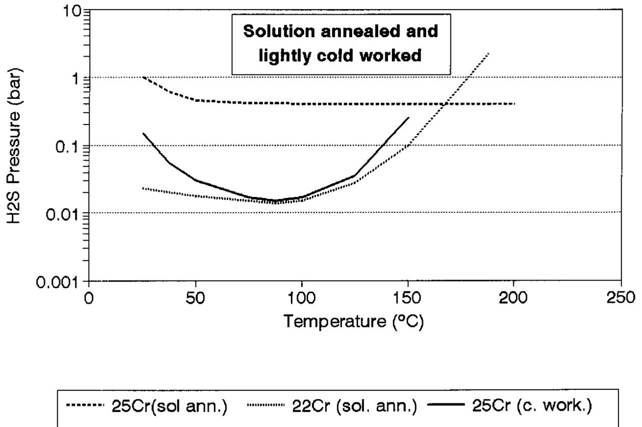
FIGURE 2 Effect of temperature on the H<sub>2</sub>S limit for SSCC for duplex (Ref 1)
